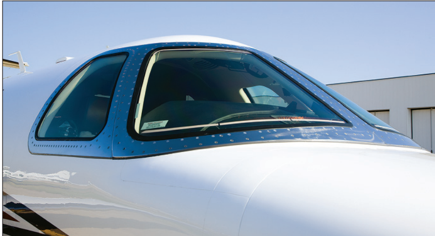
CJ4's nose has been recontoured and it features new stronger, albeit smaller, conical-section, glass windshields that enable V mo to be increased to 205 KIAS.
