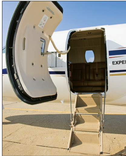
The CJ4 has a redesigned door with a constant 24-inch width and 48-inch height.
