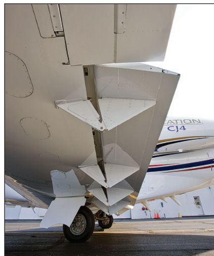
Long-span, large-area flaps assure excellent runway performance. They reflex up when retracted thereby reducing high-speed drag.
