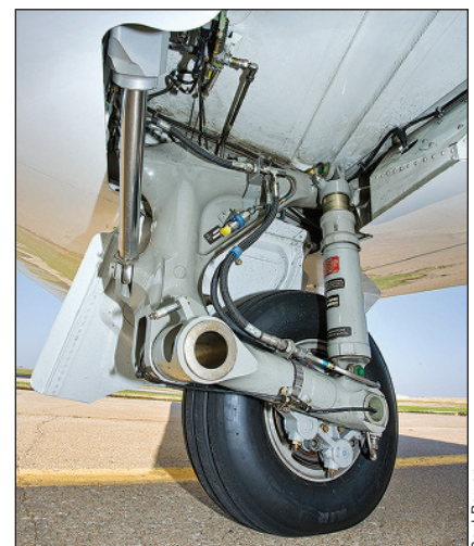
Long travel, trailing-link main landing gear assure soft touchdowns. Notably, the new wing allows optimum positioning of the landing gear.
